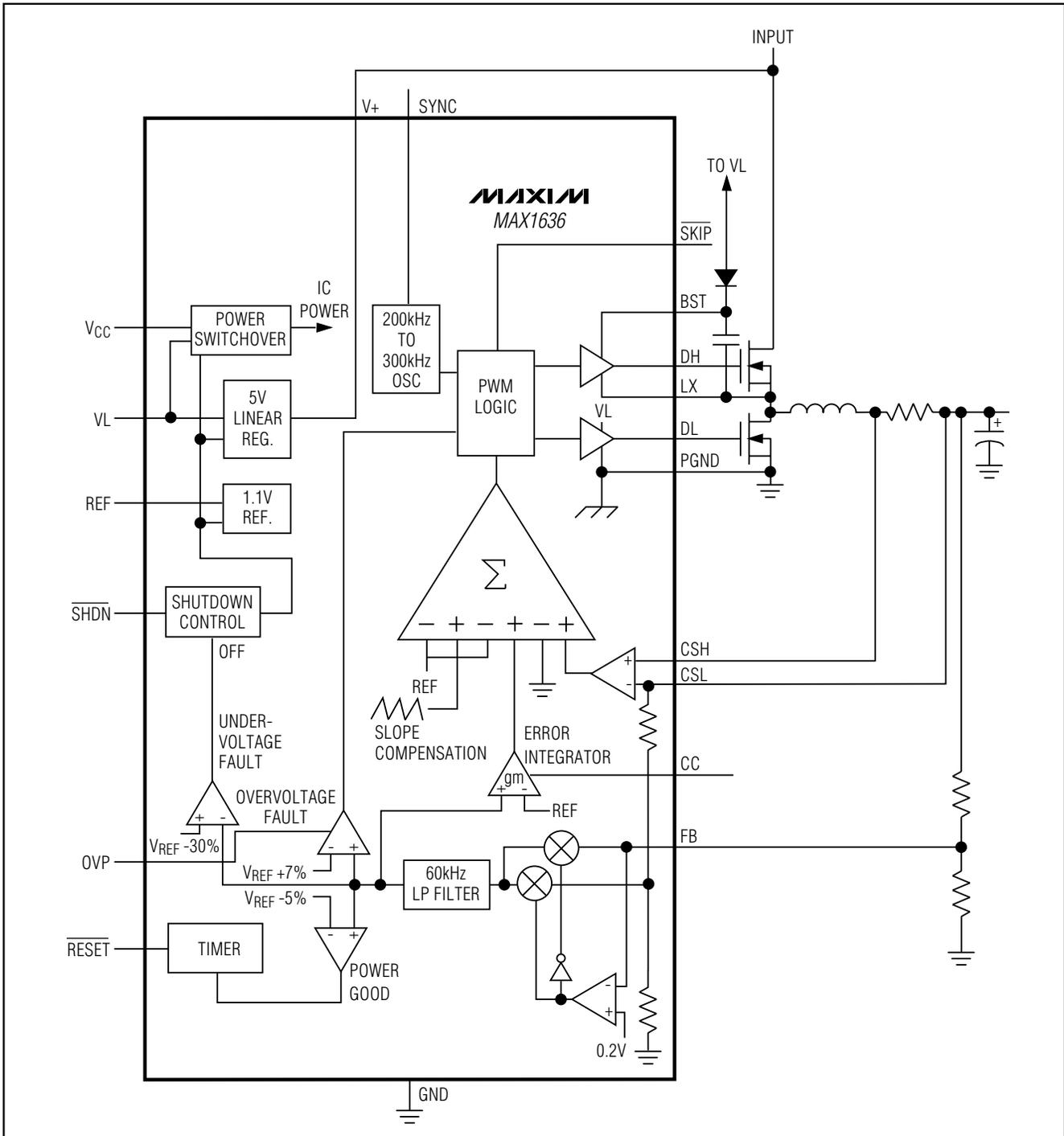
Figure 2. Functional Diagram
